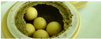
By using a ball mill, the sample will become pressed to mush within one minute. For a further grinding, it should be possible adding some solvents and receiving a homogeneous slurry / suspension.
