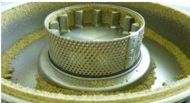
Oily sample uses to block the openings of the used 0,75mm sieve ring rapidly. A grinding of higher amounts is not possible.
