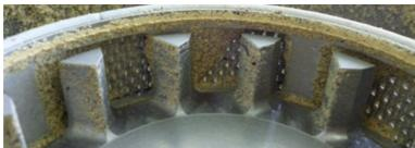
Also by using the impact bar (for temperature sensitive samples), the openings started to become closed with sample.
