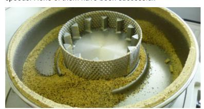
By using the 1,0mm sieve ring, all fed sample has been ground successfully. Higher amounts can be ground without problems.
